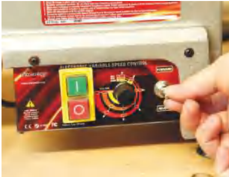
▲ The lathe is put into reverse with a simple flick of a switch
